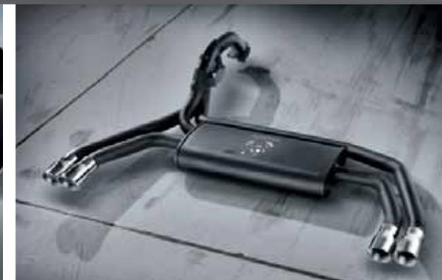
**SCARICO ABARTH RECORD MONZA.** DERIVATO DAI SISTEMI DI SCARICO ORIGINALI ABARTH E DOTATO DI TECNOLOGIA DUAL MODE. GRAZIE A UNA VALVOLA A DUE VIE A COMANDO MECCANICO POSIZIONATA IN CIMA AL SILENZIATORE PUÒ MODIFICARE LA CURVA DI COMPRESSIONE DELLO SCARICO. GIÀ A MEDI REGIMI E LA DIFFERENZA SI SENTE: LA VALVOLA SI APRE, IL SOUND DIVENTA CATTIVO E LA RISPOSTA DEL MOTORE PIÙ PRONTA. DI SERIE SU ABARTH595 COMPETIZIONE.
