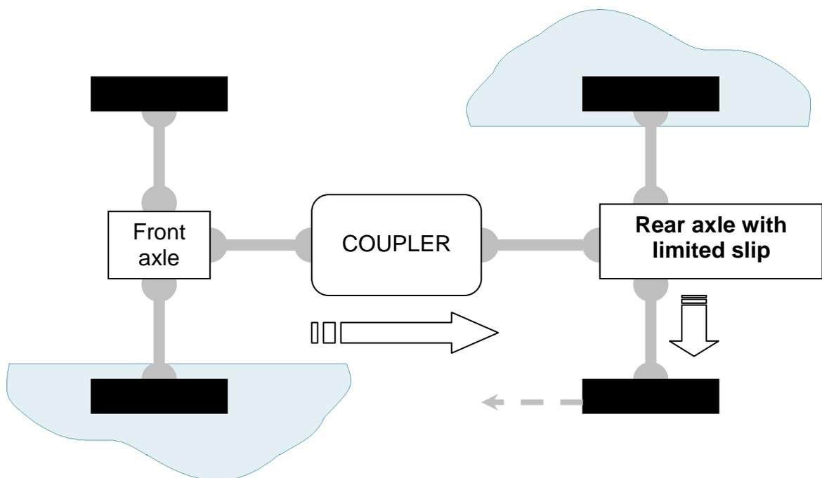
**LOSS OF GRIP OF A REAR WHEEL AND OF A FRONT WHEEL;
