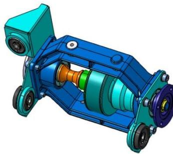
Permanently active, it detects the loss of grip of the front wheels and then transmits the engine torque to the rear wheels.
