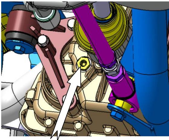
**The filling plug does not indicate the oil level**
