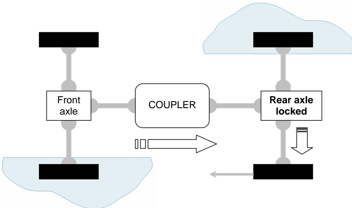
**LOSS OF GRIP OF A REAR WHEEL AND FRONT WHEELS ;
