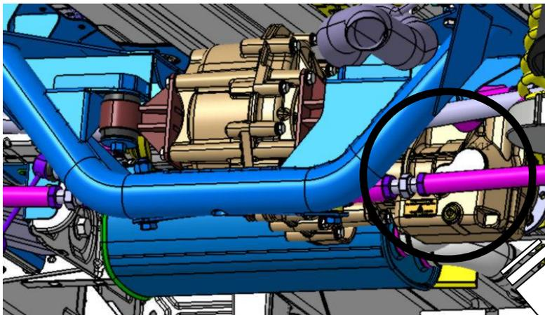
The filling plug does not indicate the oil level
